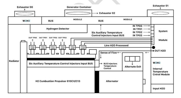
Upon a failure of the hydrogen synthesis process, **H2** inhibits hydrogen water processing and enables exhaust fans by eliminating flammable atmosphere.
