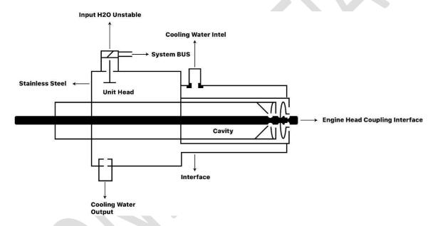
The cylindrical interface is connected to the internal combustion engine head.
